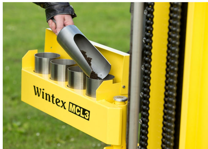
The soil is removed from the probe and filled into the soil bins with a sampling scoop and a scraper.
