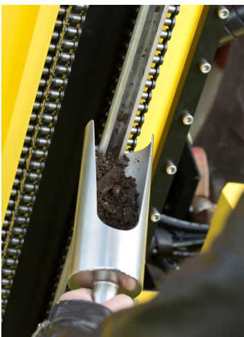
The soil is removed from the probe and filled into the soil bins with a sampling scoop and a scraper.
