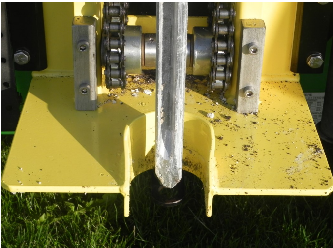
The tip of the probe is specially designed and ensures homogeneous and representative soil samples.
