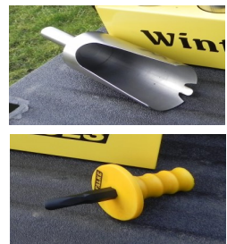
Extras: a custom-made probe with an integrated plastic liner makes it possible to extract and keep a whole core of soil.
