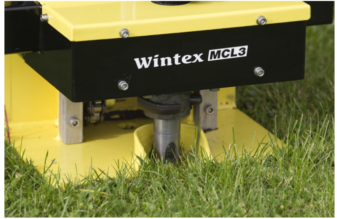
The probe goes into the ground by the means of a high-frequency hammer.
