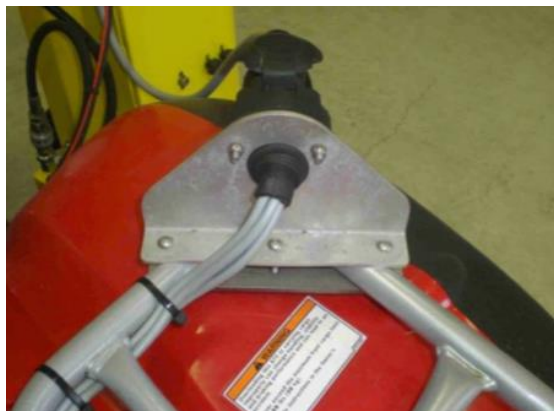
Mount the bracket for the 13-pole plug in a suitable position near the soil sampler.
