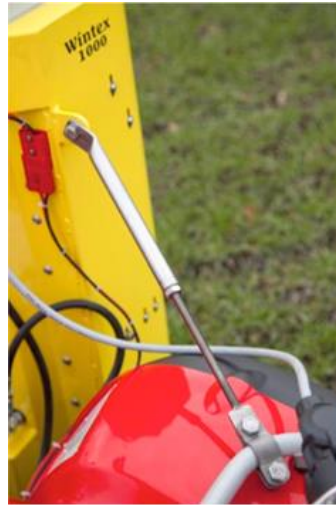
The cable with the red plug must be connected to the battery of the ATV: red +, black -.
